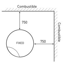
Clearances may be reduced with the application of heat shielding to walls in accordance to the Australian Building Code.
